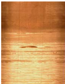
Optical image of sandstone where lower section has not been sufficiently cleaned out - resulting in a smeared borehole wall
